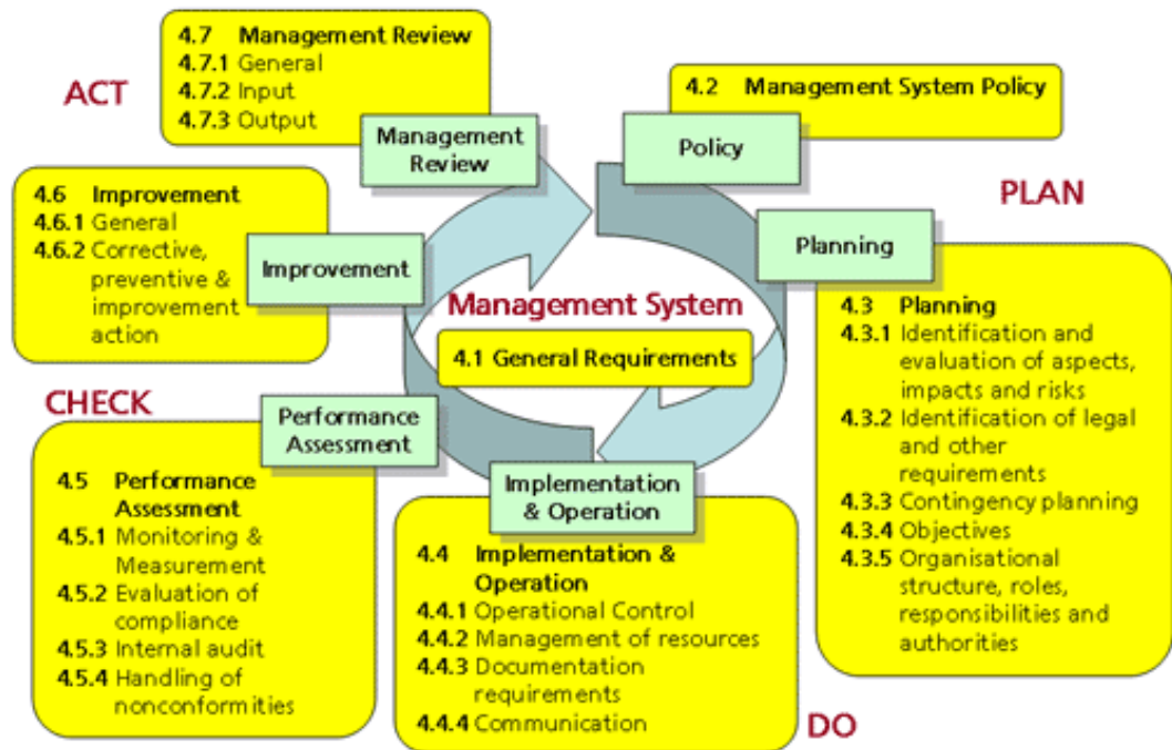
Figure 3.2 Structure of a management system according to PAS 99 and PDCA
