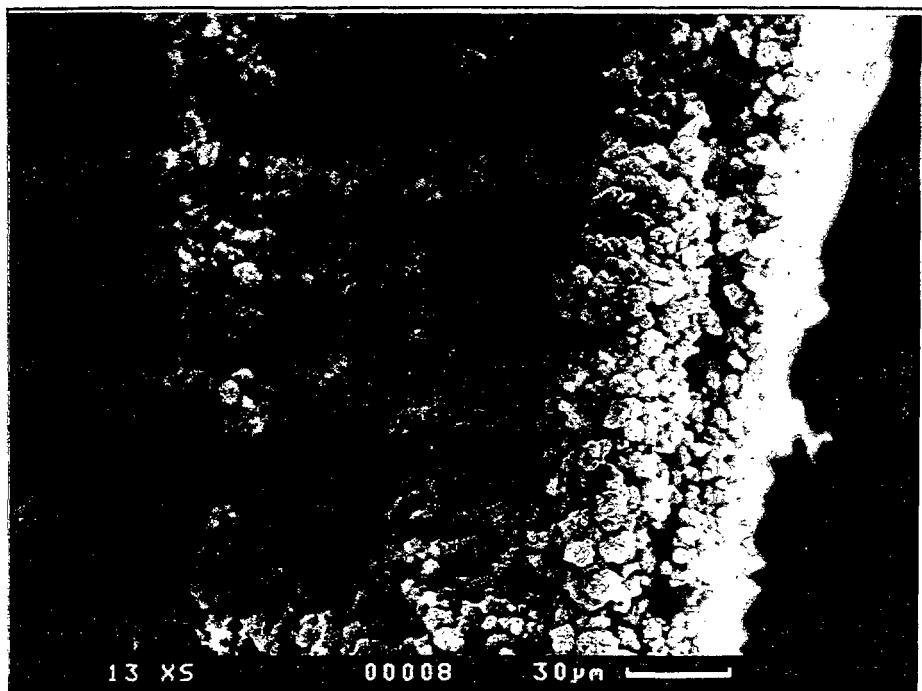
FIGURE 7: Silicon Carbide Coating Prepared by Twin Torch Plasma.
