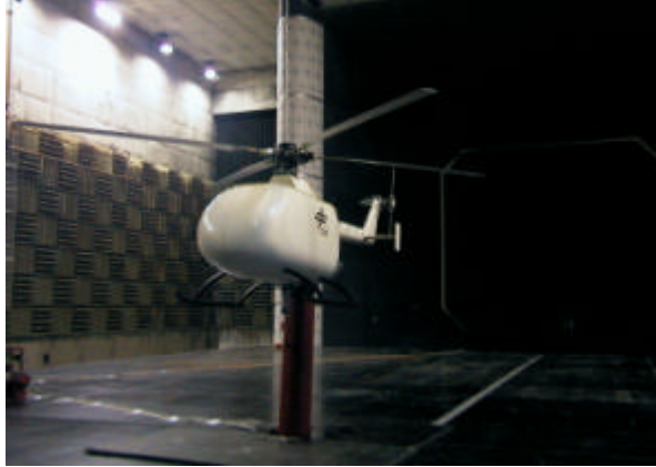
Figure 5.1: BO 105 wind tunnel model mounted in DNW open test section over a ground plane (for Task 3 tests)
