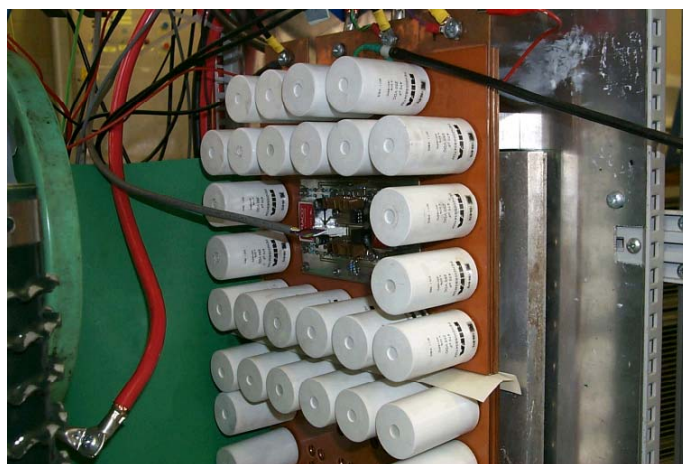
Figure 6.2. Power stage of OPTELEC brass-board dc-to-dc converter.
