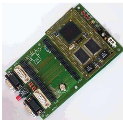
Figure 9.1. VMU hardware platform developed by Traxis for the OPTELEC project.
