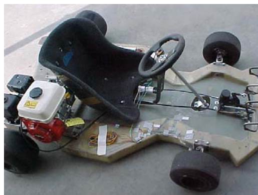
Fig.12 go-kart with strain gauges
