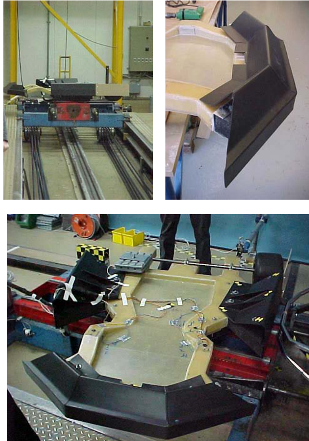
Fig. 15 side bumper impact test and bumper prototypes
