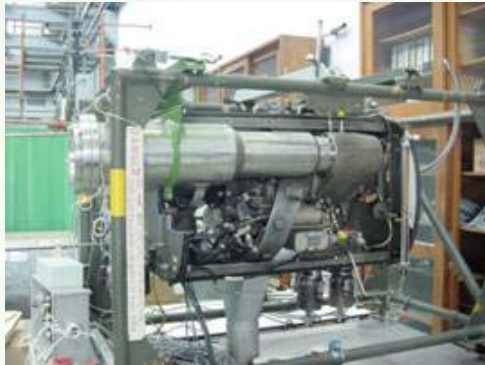
New ALSTOM Combustor installed on turbine at TUD
