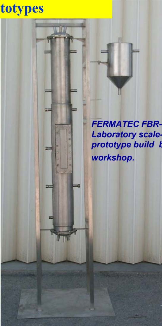
FERMATEC FBR-3P Laboratory scale-up prototype designed by Tecnia research team.
