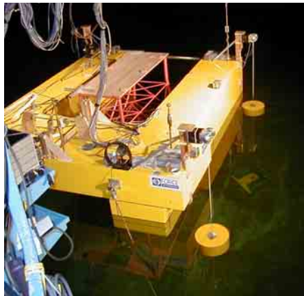
Tank model test of "Sea Fork One"
