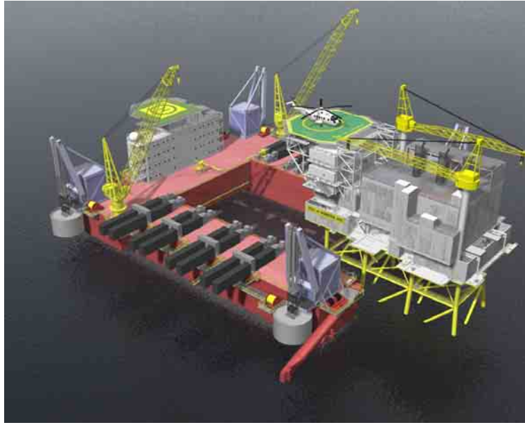
Main beams in LTS retracted during positioning
