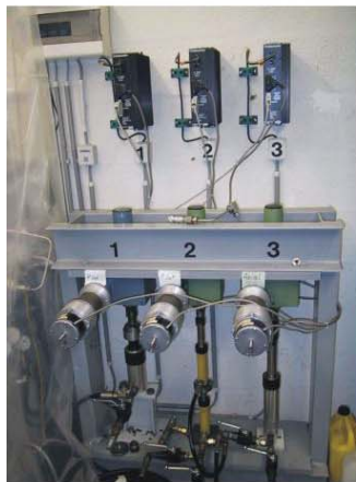
The auto-compensated suction controlled triaxial cell : general layout of the control system
