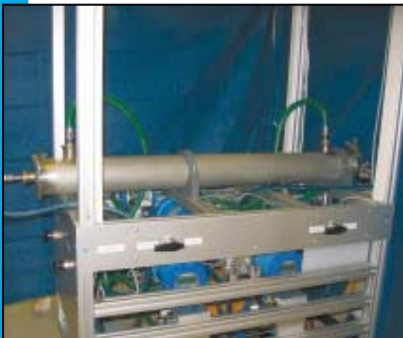
A spiral module design for pilot testing has been developed and three modules with 4 m 2 of membrane each have been produced. One of these has been in successful operation for several weeks and the power yield was as expected.
