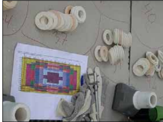
Figure 1.2-15: Ceramic orifices and installation pattern
