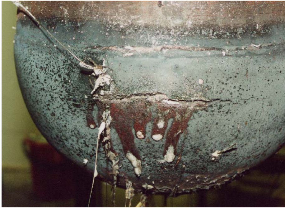
Figure 2: Post-test view of the failure site in EC-Forever-2 test.
