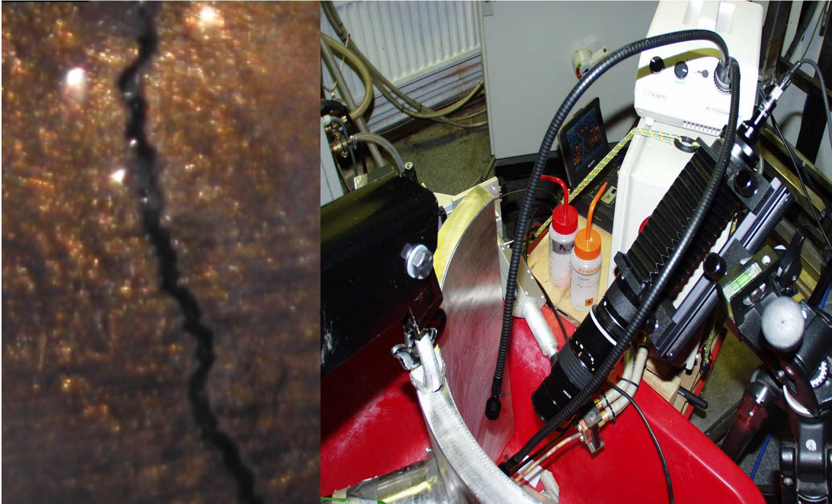
Figure 26: “Fortum train”, thermal shock experiment, crack monitoring
