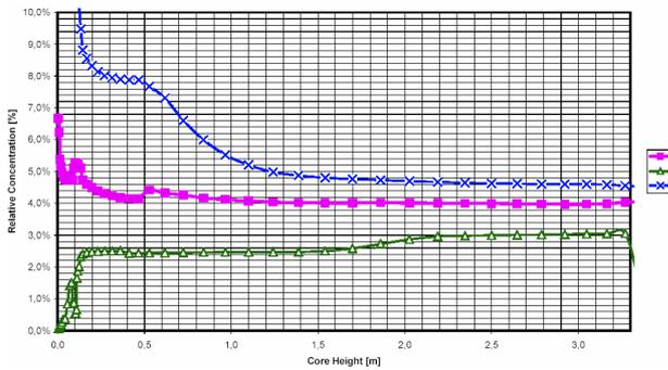
Figure 3: Relative boron concentration (mean, min., max.) across core height. Case I: injection/bypass ratio 4 %, inj. veloc./angle: 20 m/s, 40 deg.
