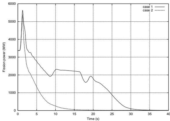
Figure 5: Fission power for the first 40 seconds in the TRAB-3D calculations
