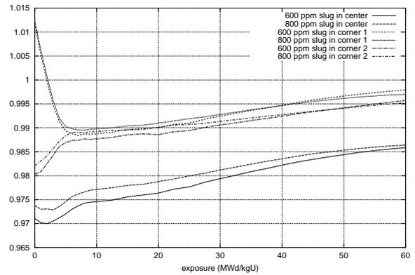
Figure 4: Boron heterogeneity weight factor for a 3 cm slug of 600 and 800 ppm boron concentration
