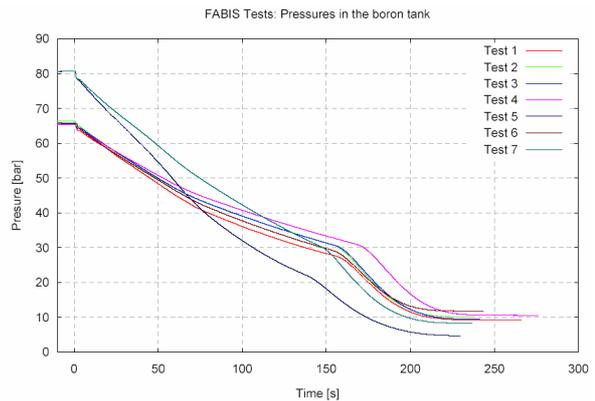
Figure 6: Depressurization of the boron tank in the experiments of WP4
