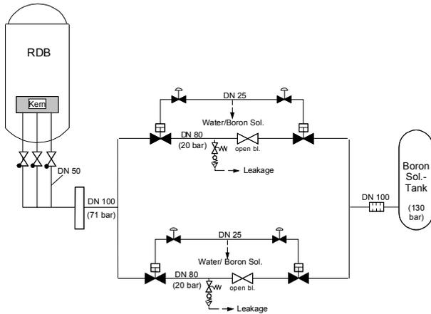
Figure 1: Principle flow diagram of the Fast-Acting Boron Injection System, FABIS
