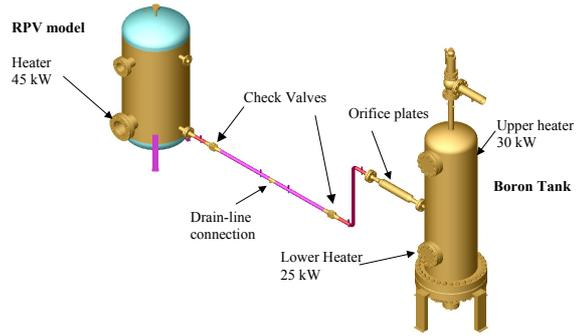
Figure 2: Principle view of the test rig of WP 4
