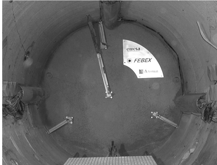
Figure 7: Final appearance of the plug with sensors for displacement tracking
