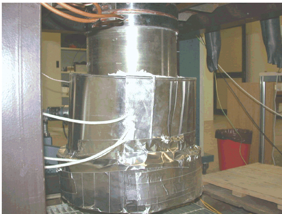
Figure 44. Detail of the thermal insulation of the ER, also showing the copper coil used for cooling
