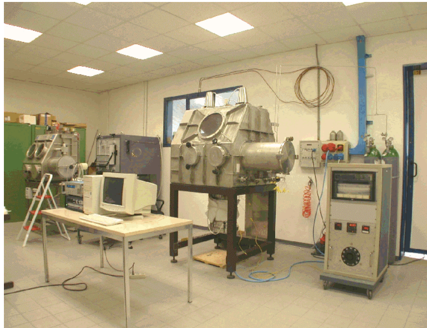
Figure 43. General view of the plant, with steel glove box, electrical supply for heating the ER, and the PC data acquisition system
