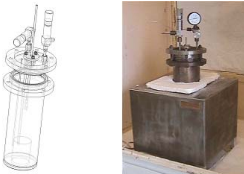
Figure 14. The prototype electrolyser: 3D drawing and final product placed in the resistance oven
