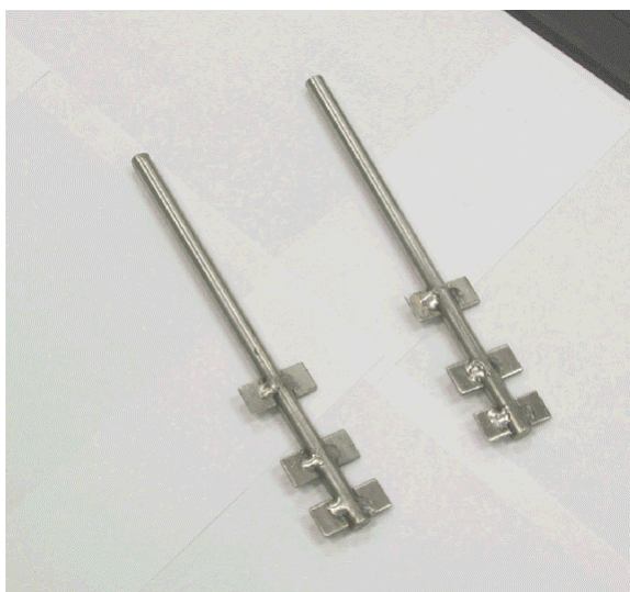
Figure 48. Pair of paddle-shaped stirrers with three baffles used for evaluating the mixing efficiency
