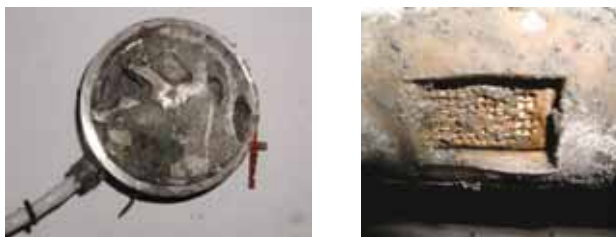
Figure 7: Chemical corrosion in a total pressure cell (left) and detail of a piezometer installed in a borehole at 0.5 m distance from the heater (right).
