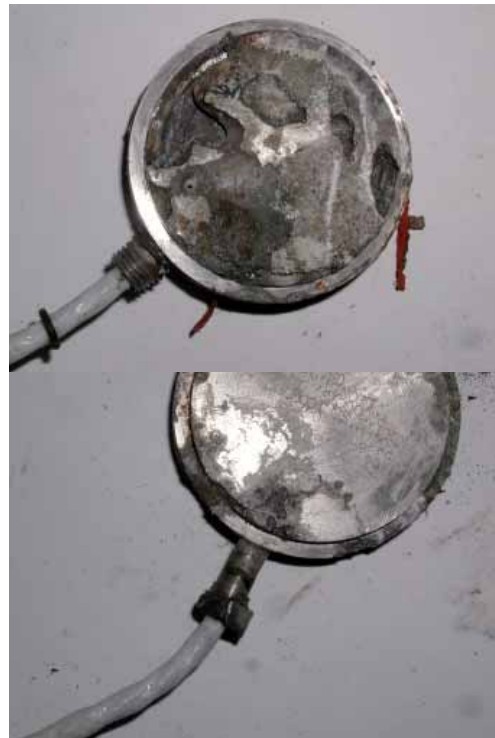
Figure 4.13: Corrosion in a total pressure cell.
