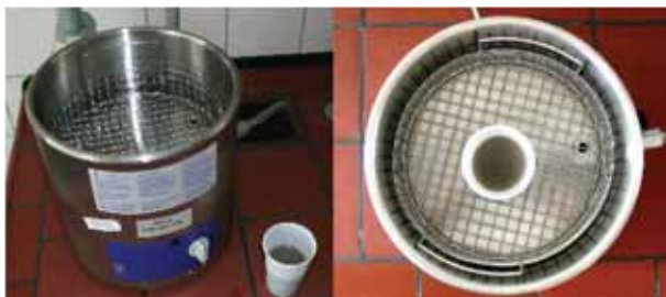
Figure 6.2: Photograph of the thin plastic cup containing the mixture of sample and water which is placed in the ultrasonic bath. The generated suspension is decanted and collected in a bucket.
