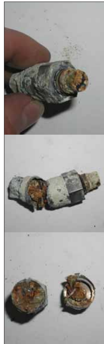
Figure 4.10: Effects of corrosion in a pore pressure sensor.
