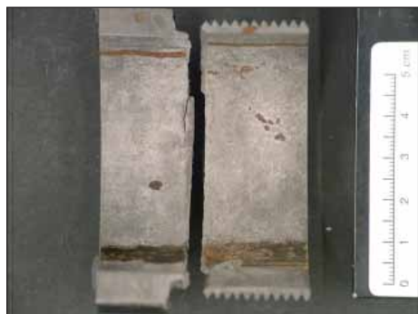
Figure 4.14: Fracture region (inside; after chemical removal of the corrosion products).
