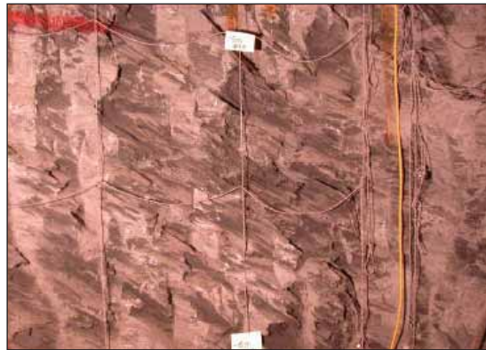
Figure 4.9: Photo taken at a depth of 6 m. The well-developed bedding leads to a strong anisotropy. side square length is 0.5 m.
