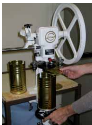
Figure 6.35 Folding machine for tin boxes with tin boxes of 113 mm diameter and 205 mm height (left). PVC liner with transport pallet of BGR liners (right).
