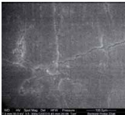
Figure 5.6: ESEM pictures of bentonite sample 22 at 40 % relative humidity (top) to 90 % relative humidity (bottom). Pictures are taken after 1 min equilibration time.
