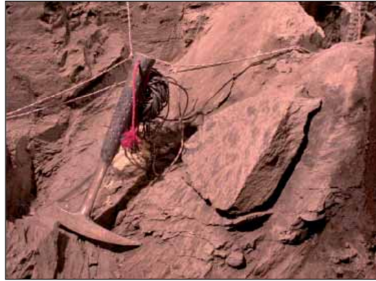
Figure 4.8: Slickensides on a fault plane (broken block). Shear sense is consistent with a thrust movement. The upper part (hanging wall) is ramped above the lower part.
