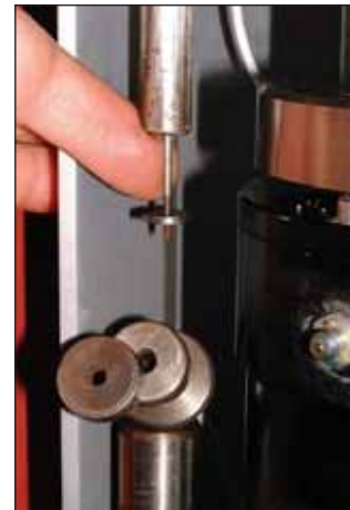
Figure 4.18: Corrosion of laboratory equipment exposed to Opalinus Clay samples.
