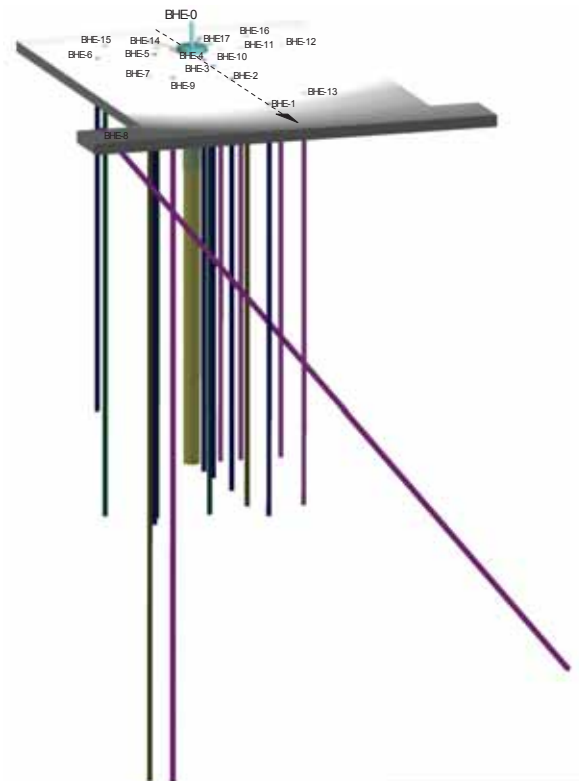
Figure 2.5: Three-dimensional (3D) view of HE boreholes.
