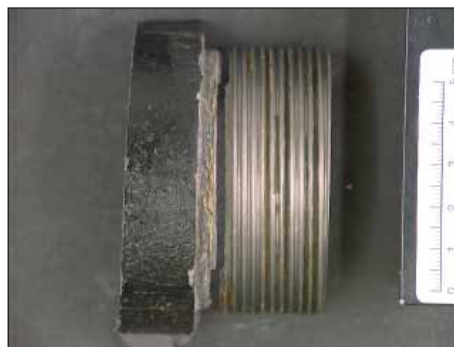
Figure 4.15: Fracture region (outside; after chemical removal of corrosion products).
