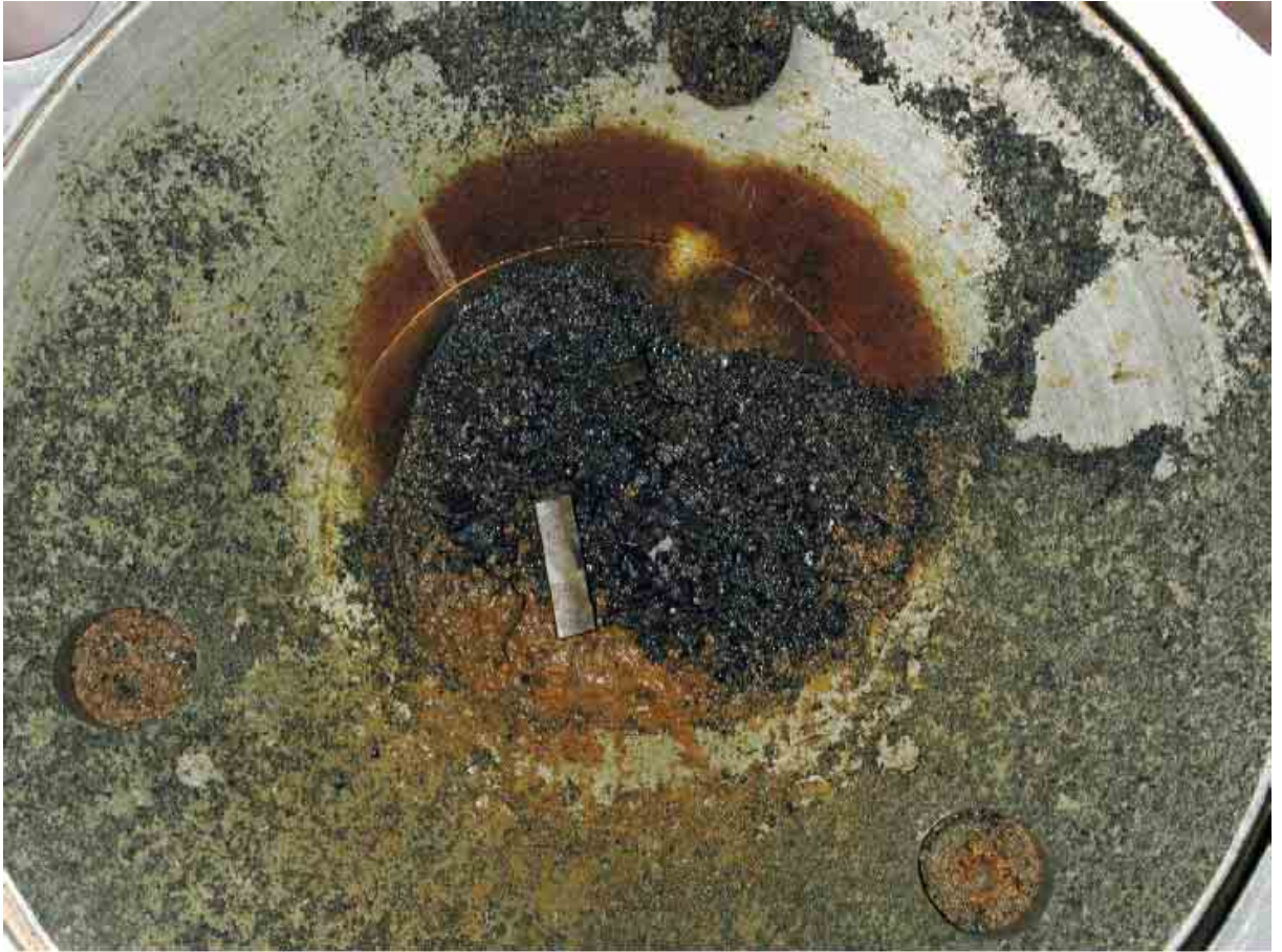
Fig. 37: Post-test examination of the test section (after drainage of the water)
