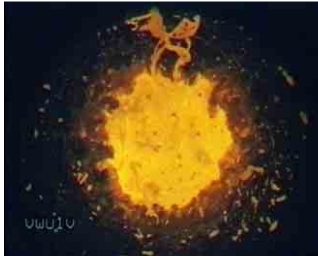
Fig. 20: Corium pool agitated by the steam flow from bottom flooding in the COMET cooling device
