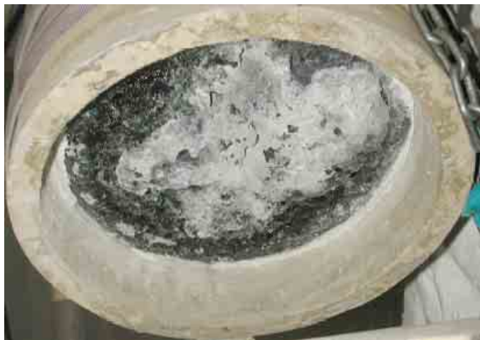
Fig. 30: Bottom view of the corium pool after the zirconia crucible has been removed from the COMET core-catcher
