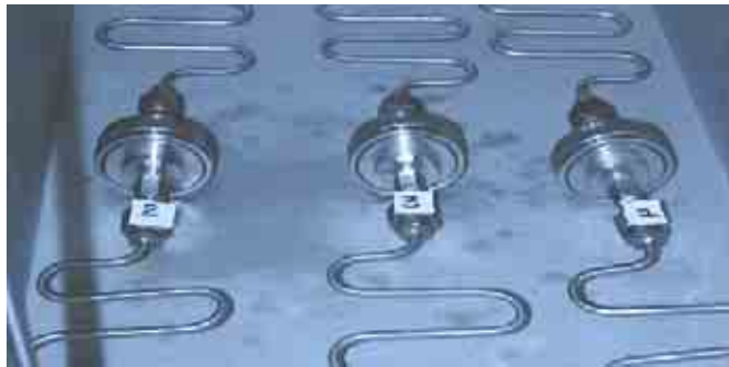
Fig. 4: COLIMA aerosol filter lines
