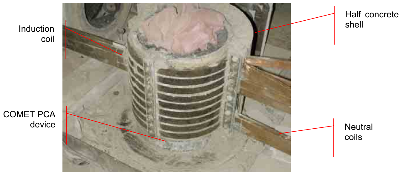
Fig. 27: After sawing half of the concrete shell
