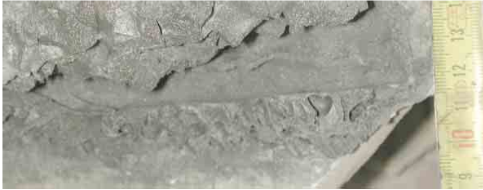
Fig. 31: Chimneys observed at the lower part of the corium pool
