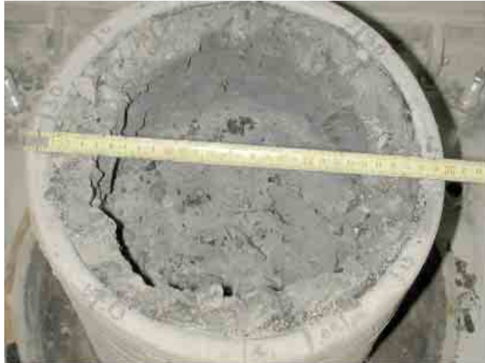
Fig. 29: Top view of the corium pool in the zirconia crucible
