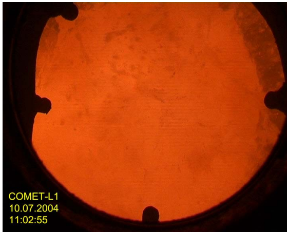
Fig. 25: Interaction of melt and concrete in the beginning of the test
