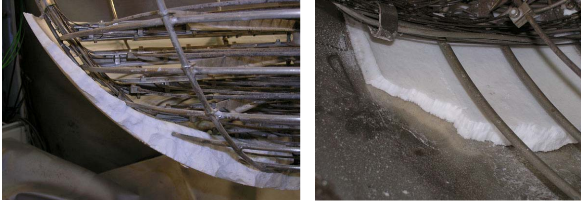
Fig. 65: Crust formed during the LIVE-L1 test
