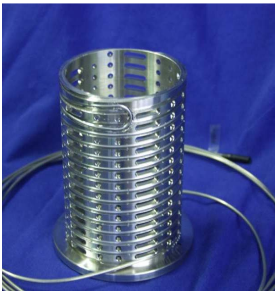
Fig. 10: Stainless-steel auxiliary heater
