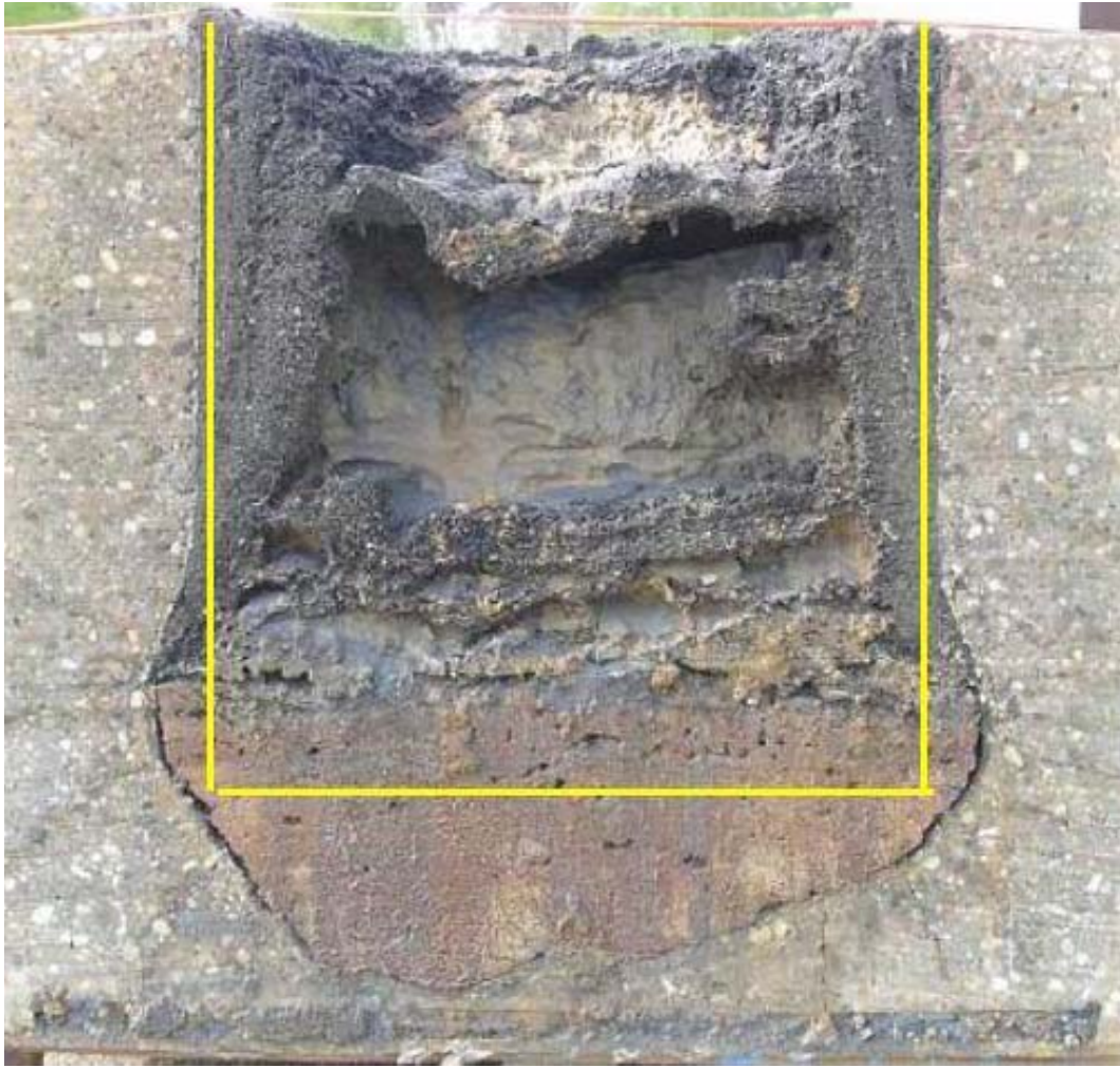
Fig. 36: Eroded concrete crucible
