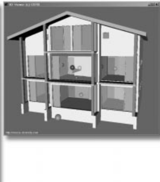
The acoustics application positions a listener in the building and simulates the effect of the surrounding sounds
