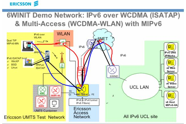
A simulated ambulance professionals communicate via a mobile terminal, capable of providing voice, video and data on body parameters from a patient like electro-cardiograms and blood pressure, communicate via both a UMTS test cell and a wireless LAN with other professionals in a simulated hospital. The communication uses Mobile IP and simultaneous multi-access, with secured data transmission based on a Public Key Infrastructure.
