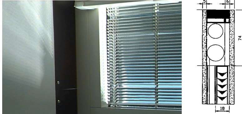
Figure 1 + 2: Light guiding property and section of the "Fish" System
