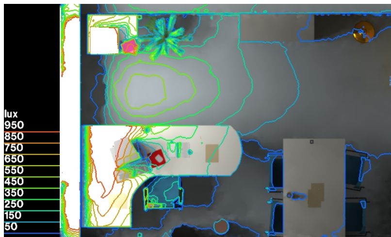
Figure 4.7.10: Top view with illuminance distribution during day (only daylight: overcast sky) for the Eindhoven test offices
