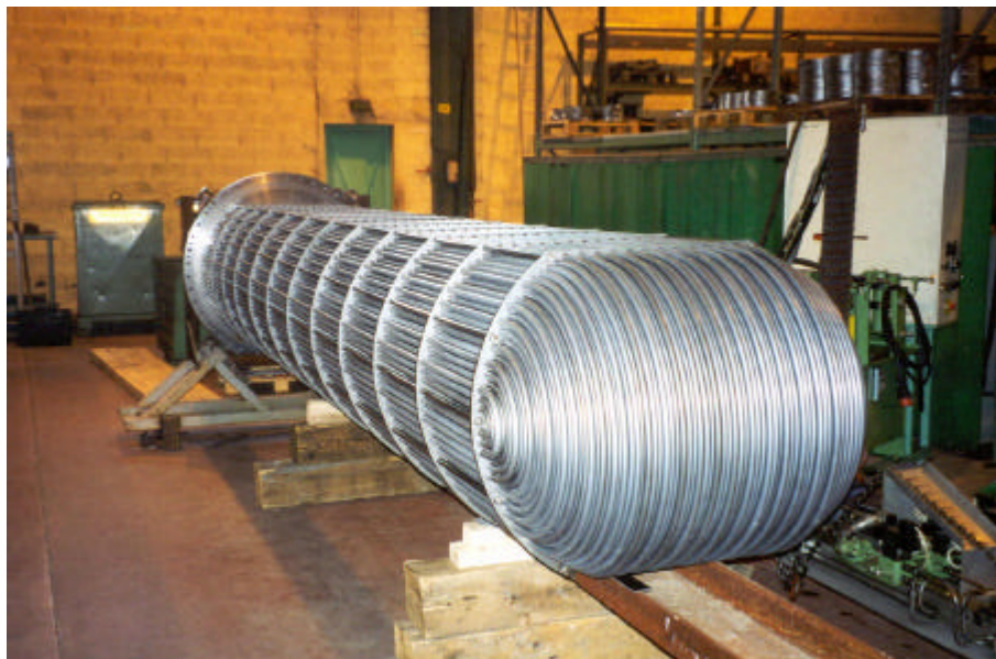
Figure 4: Bundle during construction (CIAT factory)
