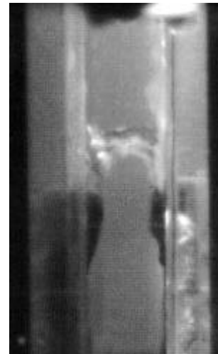
Fig. 4. The "wave bridging" mechanism. View between the plates, inside the 10mm gap.
