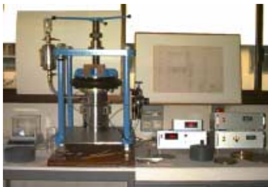
Figure 3 – Schematic description and picture of web permeameter equipment
