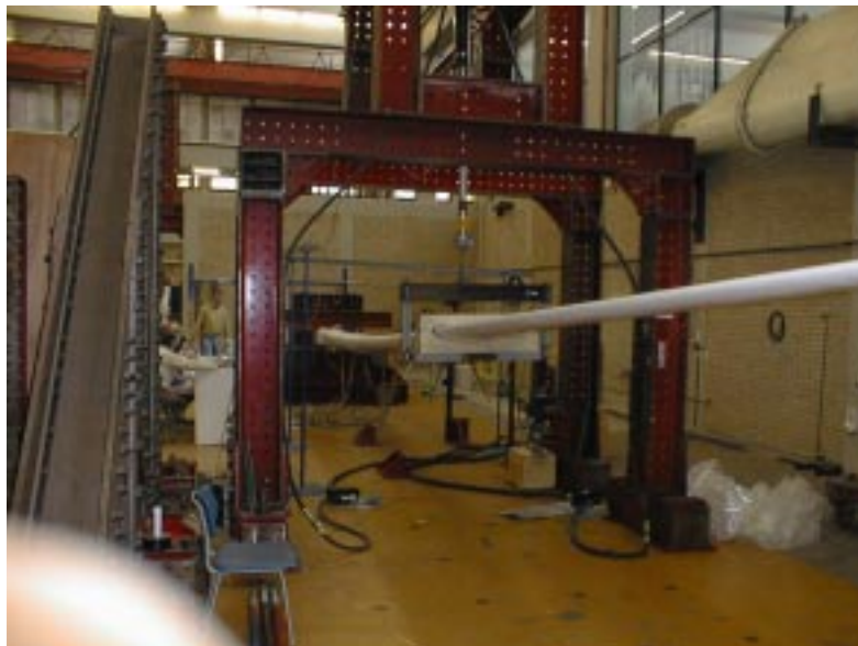
The LW30/250 blade loaded during the fatigue test
