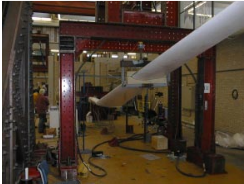
Blade failure at 125% loading during residual strength test
