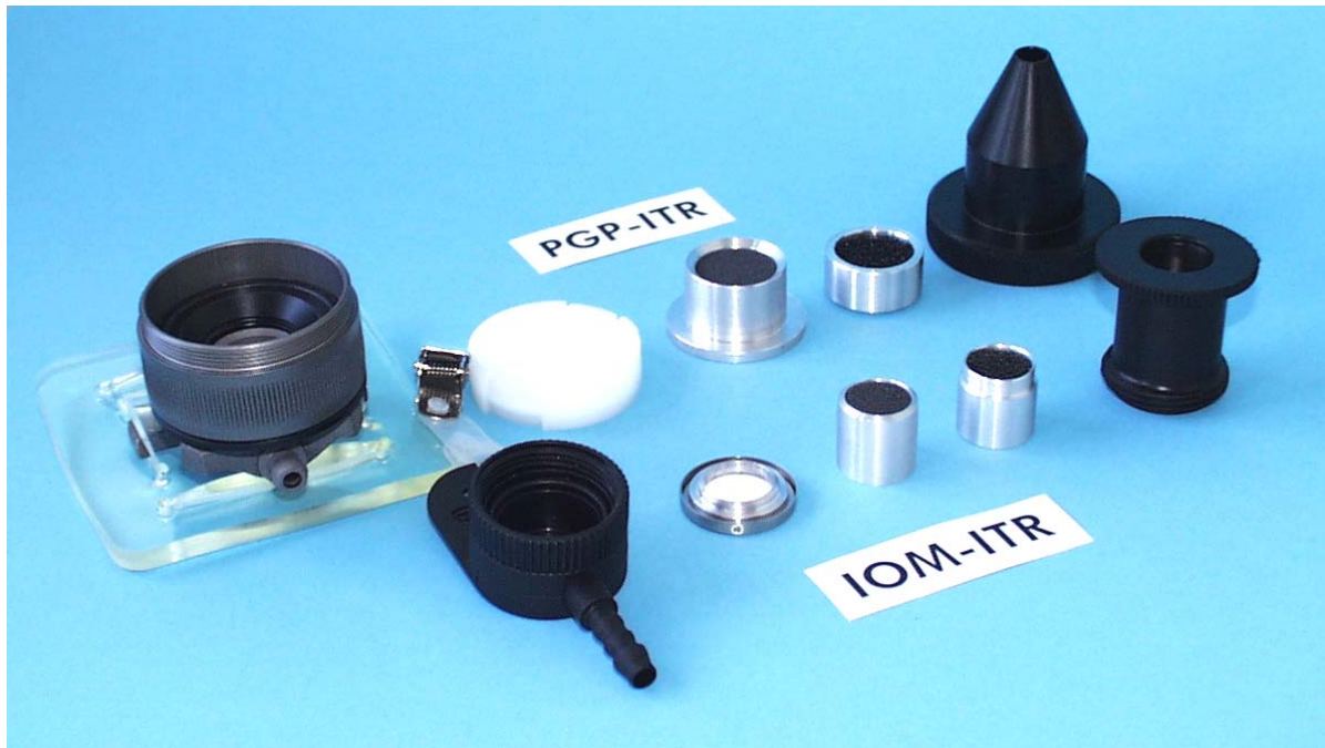
Figure 7: Prototypes for three-stage dust samplers: IOM-ITR in front row and PGP-ITR in back row.
