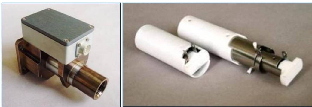
WP 2 - Figure 5 - Conductivity and capacitance sensors developed by IoA.
