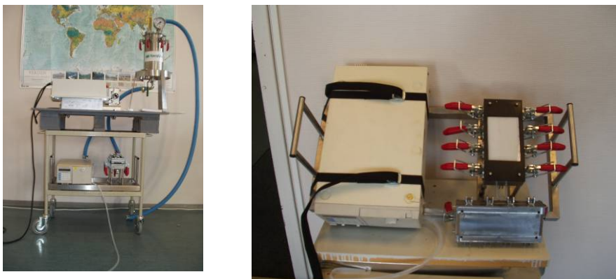
Figure 12 and 13. Images showing the pilot scale mobile membrane emulsification unit. The membrane is shown on the right figure.
