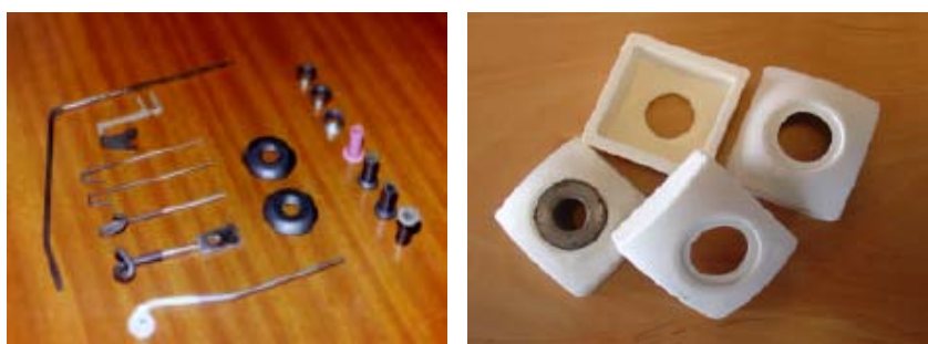
Figure 1. Some examples of applications of (A) \text{Al}_2\text{O}_3 -13wt% \text{TiO}_2 and (B) \text{ZrO}_2 -20wt% \text{Al}_2\text{O}_3 systems
