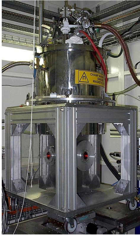
Figure 9 Cryomagnet system in operation for GINRS measurements at ID22N. The system is top-loading (up to 48 mm sample diameter). Temperatures between 1.5 and 300 K and external magnetic fields between 0 and 6 Tesla in the horizontal plane, parallel and perpendicular to the synchrotron beam, are accessible. The system is mounted on a two-circle element to allow for \Theta - 2\Theta scans of thin films and multilayers.
