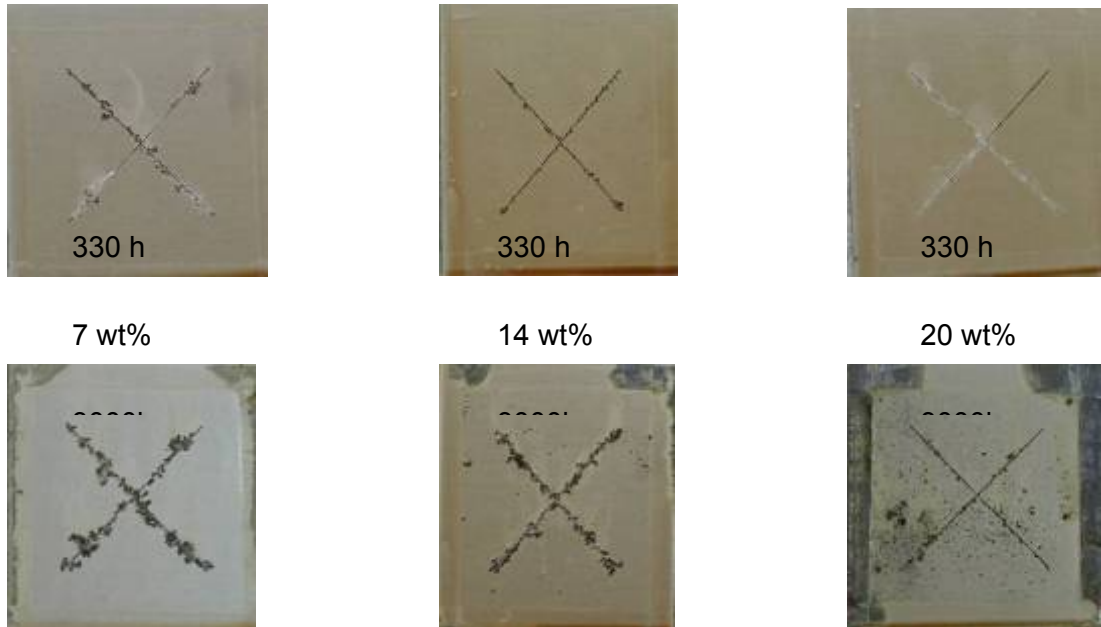
Figure 15: Epoxy based sol-gel lacquer with Cerium dioxide nanoparticles (7, 14, 20 wt%) after neutral salt spray test on aluminium alloy 2024: barrier - creepage behaviour depending on nanoparticle load of the coating (image courtesy of INM).
