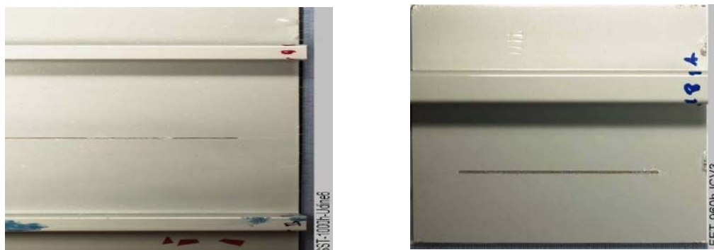
Figure 6: Left: ZrO 2 thin films with an epoxy topcoat after 1000 h in SST (Udine); Right: Macroscopic picture of glass-like Ce coating with epoxy based topcoat onto AA2024 after 960 h of Filiform Corrosion Test (ICV). (image courtesy of EADS)
