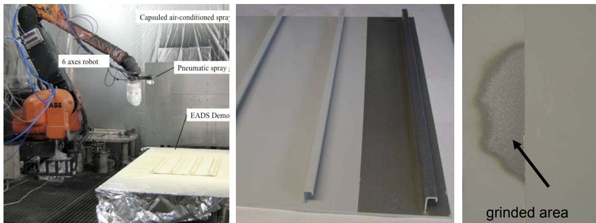
Figure 5: Left: Spray application system at IPA (image courtesy of Fh-IPA); Middle: Skin sheet of aircraft (800 x 600 mm x 3,5 mm, Material 6061, welded stringers, challenge: Homogeneous, uniform coating even on difficult to access areas (lower side of stringer) (image courtesy of EADS); Right: Sol Gel system used for repair investigation: (image courtesy of EADS)
