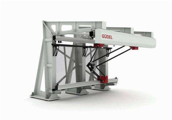
Figure 1: New parallel kinematic machine (PKM)
