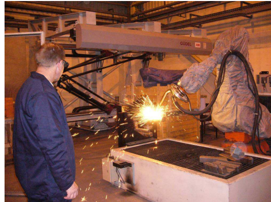
Figure 28: D1 the oxy-fuel cutting robot
