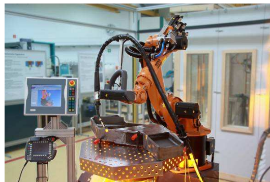
Figure 4: Programming through Manual Guidance and Graphical Post Processing
