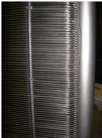
Close-up of precool matrix/header brazed joint
