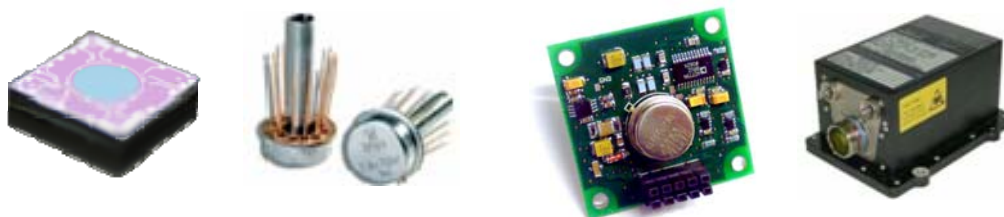
Figure 2 Development in the different work packages (sensing element, sensor package, transducer and air-data unit)
