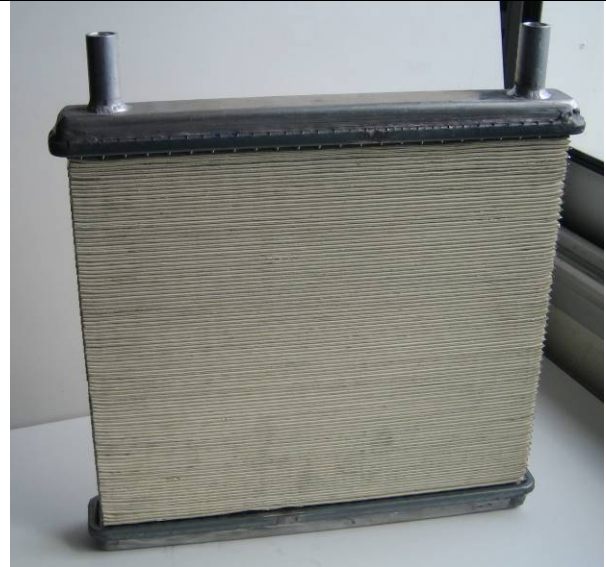
Fig. 23 Second prototype of exchanger with sorbent sheet material
