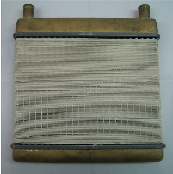
Fig. 22 First prototype of exchanger with sorbent sheet material
