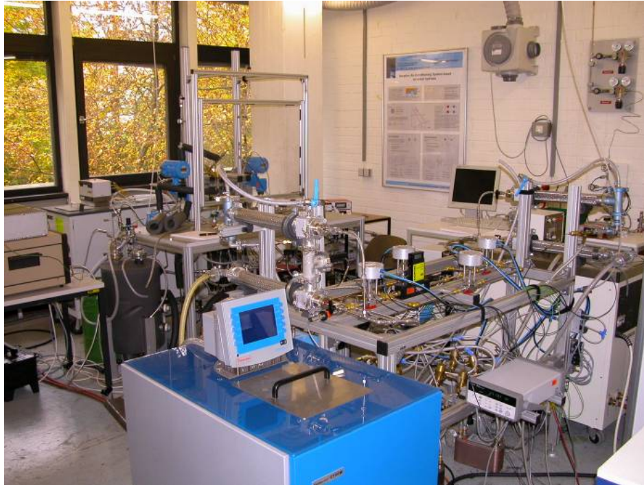
Fig.44 Picture of mechanically driven (foreground) and thermally driven (back) test benches
