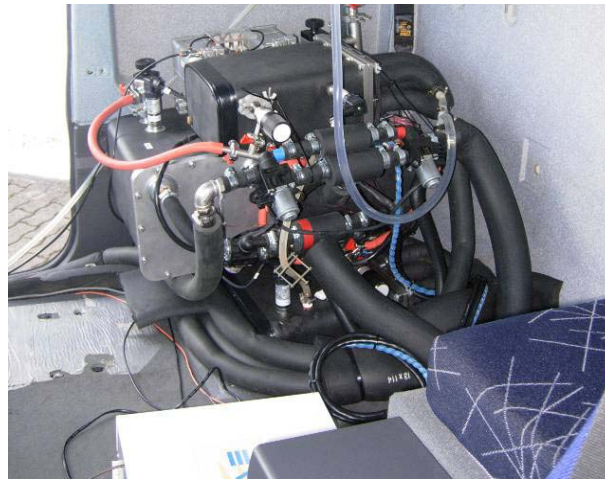
Fig.8 The adsorption chiller installed in the rear part of the cabin.
