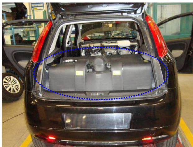
Fig.14: The prototype adsorption cooling system installed in the trunk of the Fiat Grande Punto.
