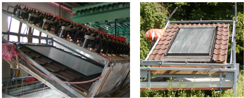
Figure 7.17 Indoor (artificial heating) and outdoor (natural heating) test facility for durability tests
