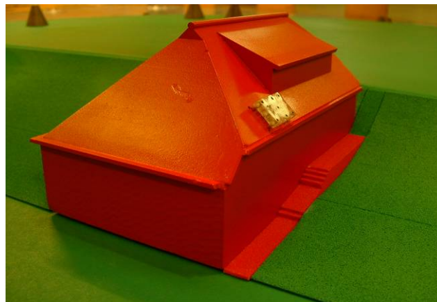
Figure 5.2: Wind tunnel model of the 'dike' house in The Netherlands
