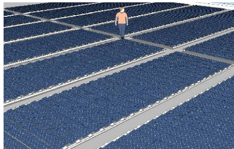
Figure 4.18: PV solution for flat roofs which utilize up to 80 % of the available roof area as PV area.
