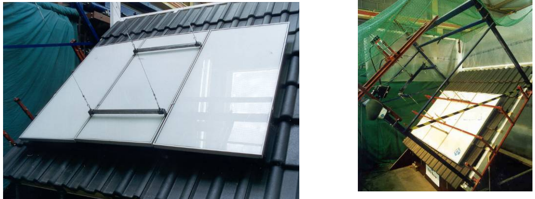
Figure 5.5 Dynamic wind load indoor test facility
