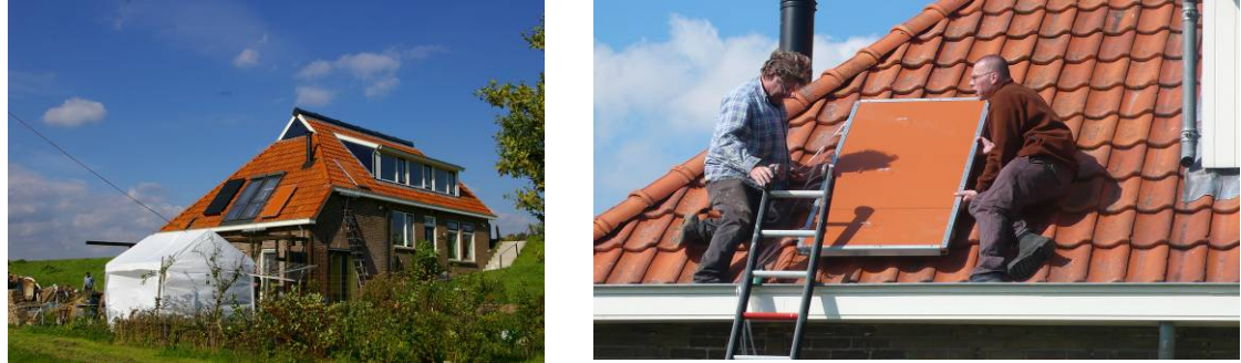
Figure 5.3 Test house and installation of the PV dummy for the wind load tests
