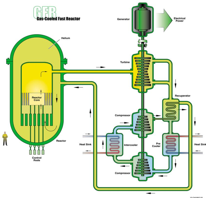
Figure 1 Gas-cooled fast reactor with a direct-cycle helium turbine for electricity production
