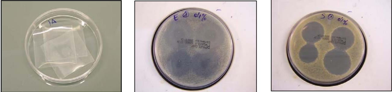
(left) Films samples for the antimicrobial activity tests; (medium) Triclosan at 0,1% (w/w) in H 2 O. Antimicrobial activity test against Escherichia coli; (right) Triclosan at 0,1% (w/w) in H 2 O.
