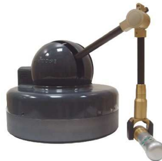
Fig. 6.b: Virtuose 3D 15-25 haptic arm developed by Haption, a CEA spin off; it provides 6 axis control and implements force feedback on 3 of them.
