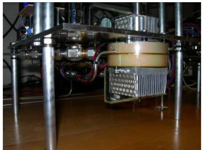
Figure 1. The Stand-Alone, Automatically Operating, Software-Controlled Laboratory Prototypes Capable of OTR Testing with Superior Sensitivity.
