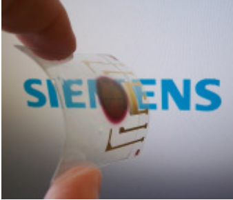
a) Fully flexible OPD with quadrant sensor layout
