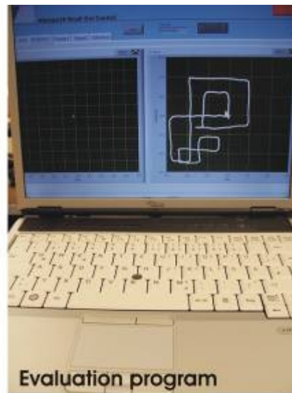
Figure 62. a) Picture of the 4-quadrant positioning demonstrator setup. b) On the screen of the PC it is possible to follow in real time the position of the spot.
