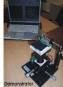
c) Demonstrator with integrated OLED and OPD for position-sensitive sensing
