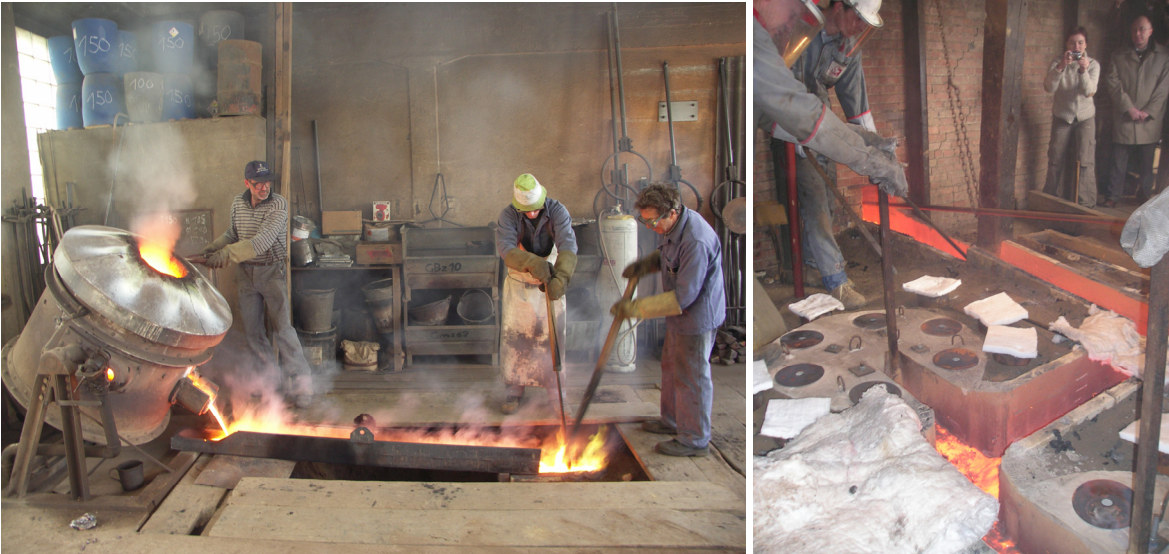
Fig. 4 Casting of bells for PROBELL Rüetschi and Cornille Havard
