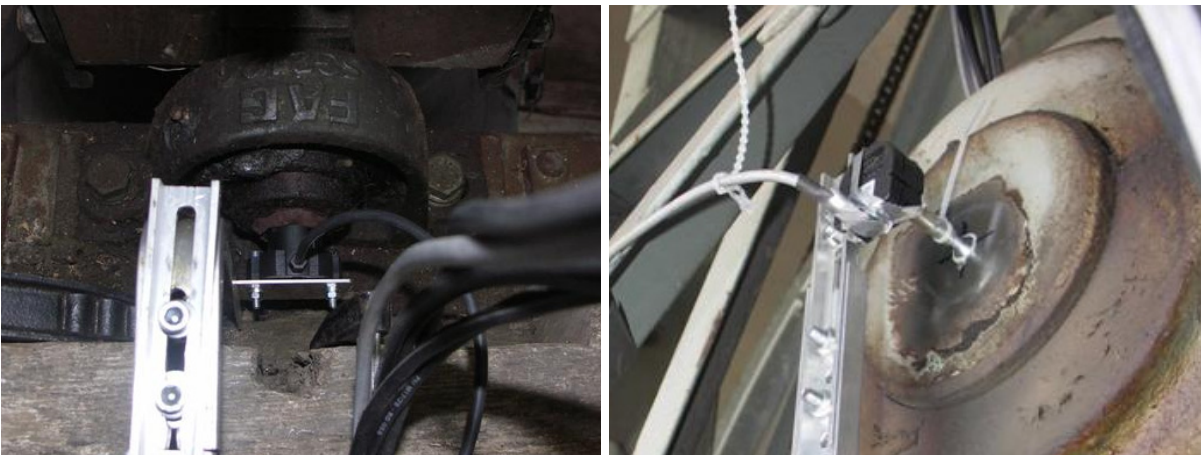
Fig. 16: Angle sensors at the rotation axis of bells
