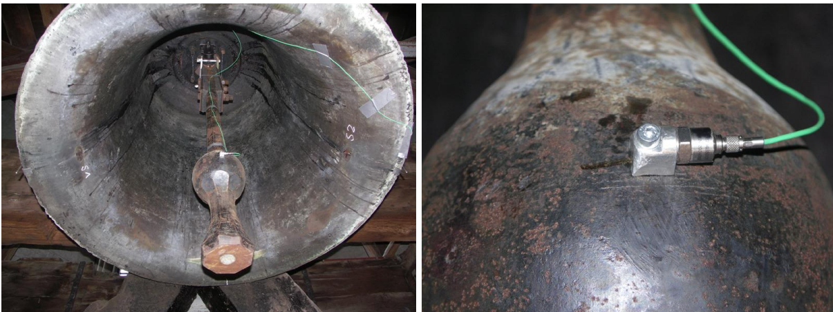
Fig. 11: Setup of accelerometer on clapper inside bell
