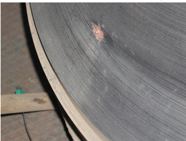
Fig. 3: Location of thermo couples
