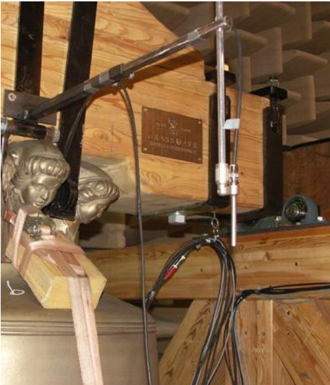
Fig. 14: Microphone (MIC Y) on the yoke of bell
