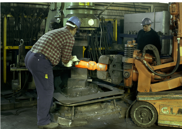
Fig. 9: Forging of PROBELL clappers at Rosswag
