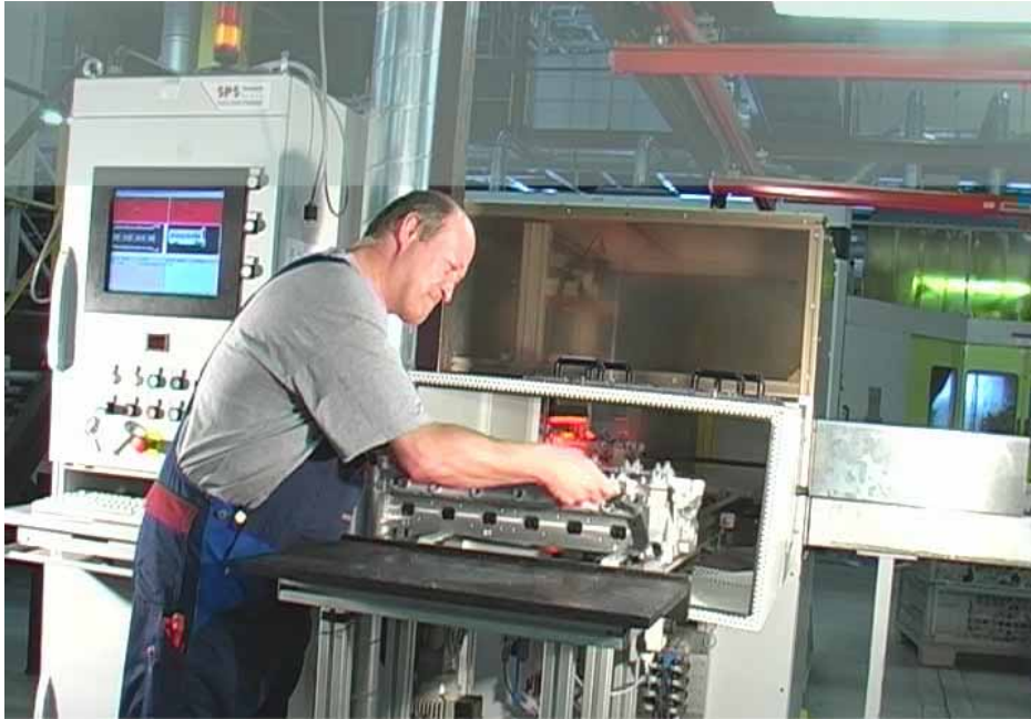
Figure 1: Visual inspection of die-cast parts.
