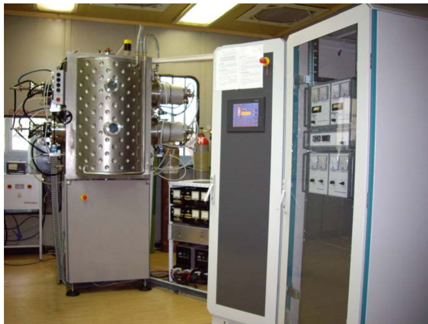
Fig. 9. Photography of the PVD equipment adapted for R&D and semi-industrial applications.
