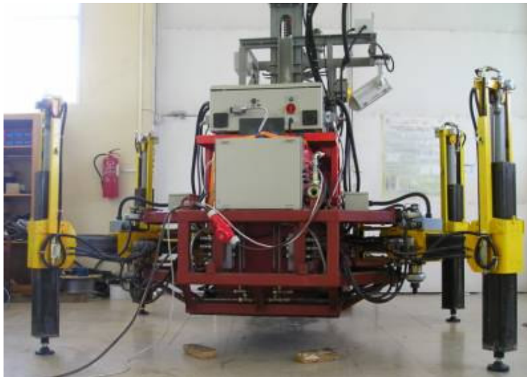
Figure 43: Integration of drilling module, legged platform and control system
