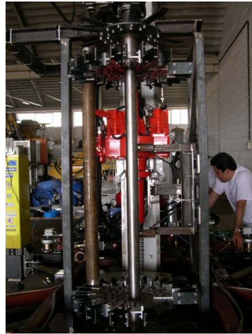
b) Rod warehouse module development
