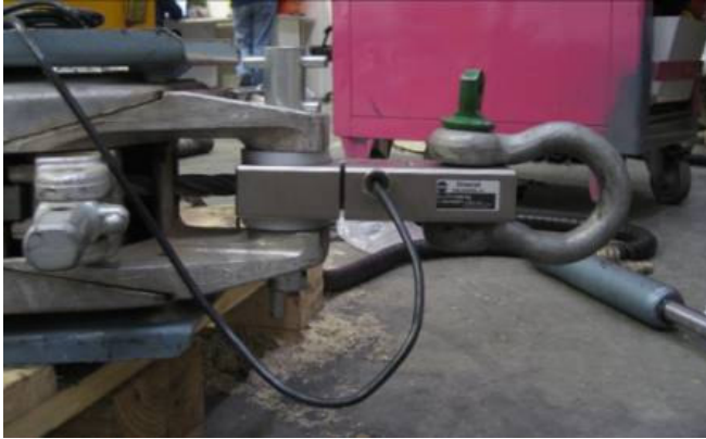
Figure 45: integration of digital strain-gauge
