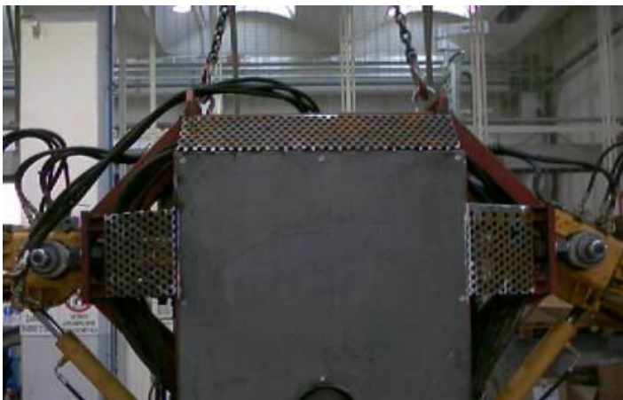
Figure 47: additional shield to protect the legs
