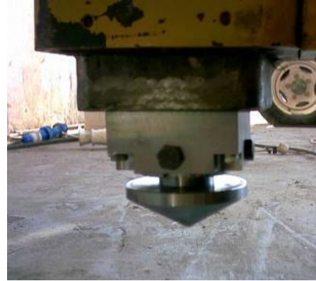
Figure 46: new foot for the robotic legs
