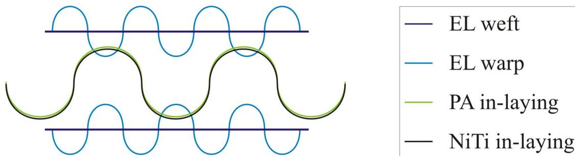
Figure 3: Loose&Tight Hybrid Textile Structure
