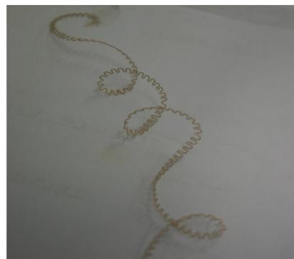
*Figure 2: Shape set hybrid NiTi/PA yarn*
