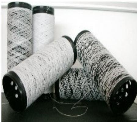
*Figure 1: Hybrid coretwist NiTi yarn*
