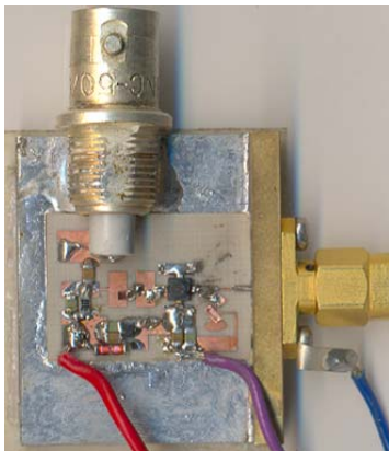
Figure 5: FET based microwave mixer
