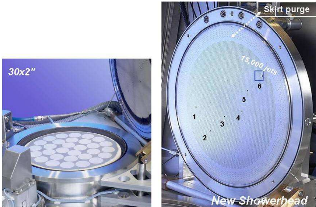
Fig. 27: Production type CCS MOCVD Reactor CRIUS in its 30x2-inch configuration.
