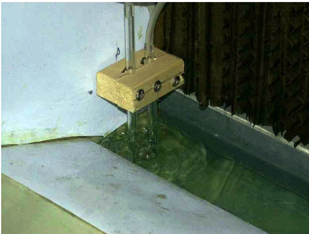
Figure 67: Measuring glass pipes in weak desiccant basin. Some bubbles are visible.
