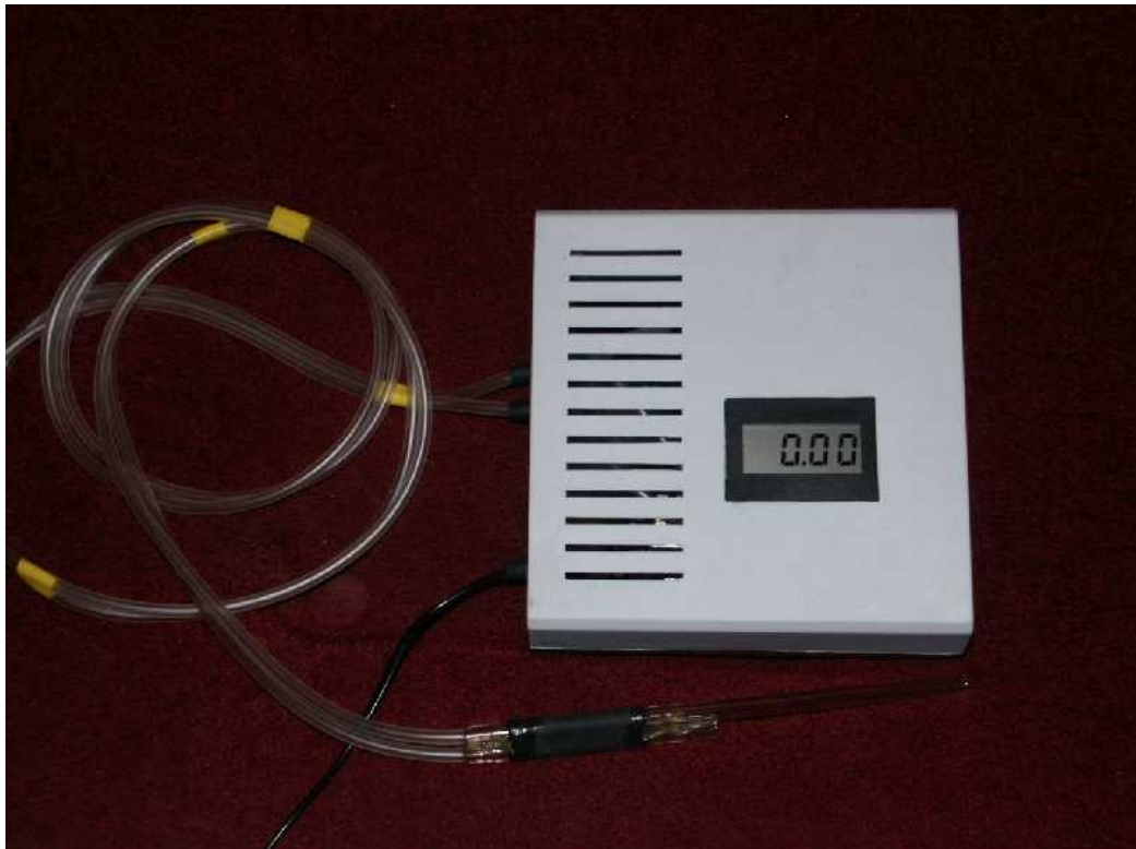
Figure 15: DM model with measurement glass pipes. The reading is equal to density in \text{g/cm}^3 .
