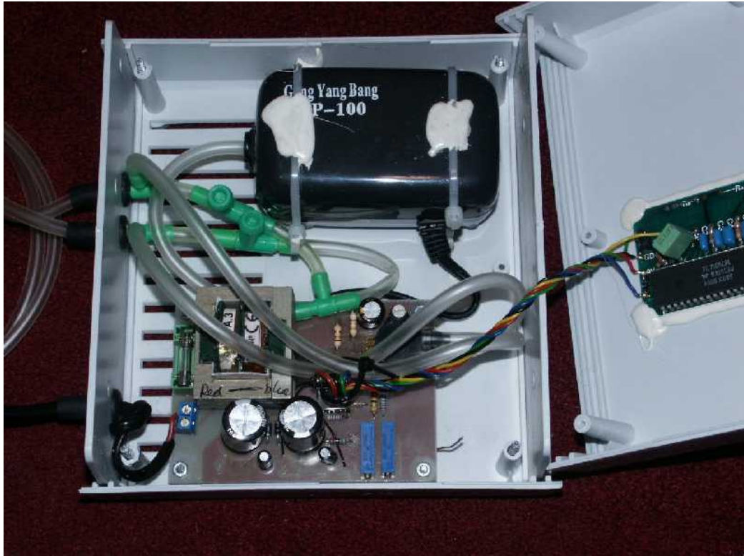
Figure 14: Density meter model with voltmeter module connected (right).
