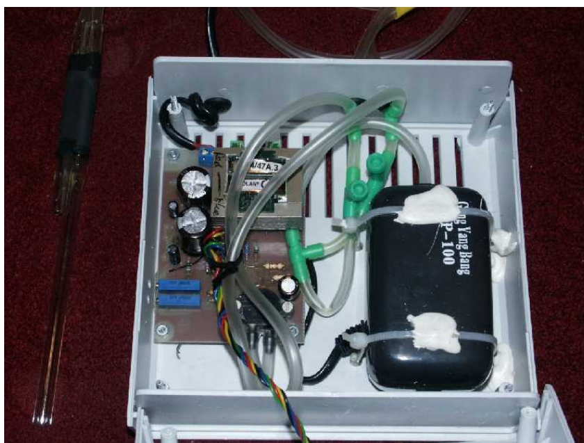
Figure 13: Density meter model. right, the air pump, left, board with electronic elements.
