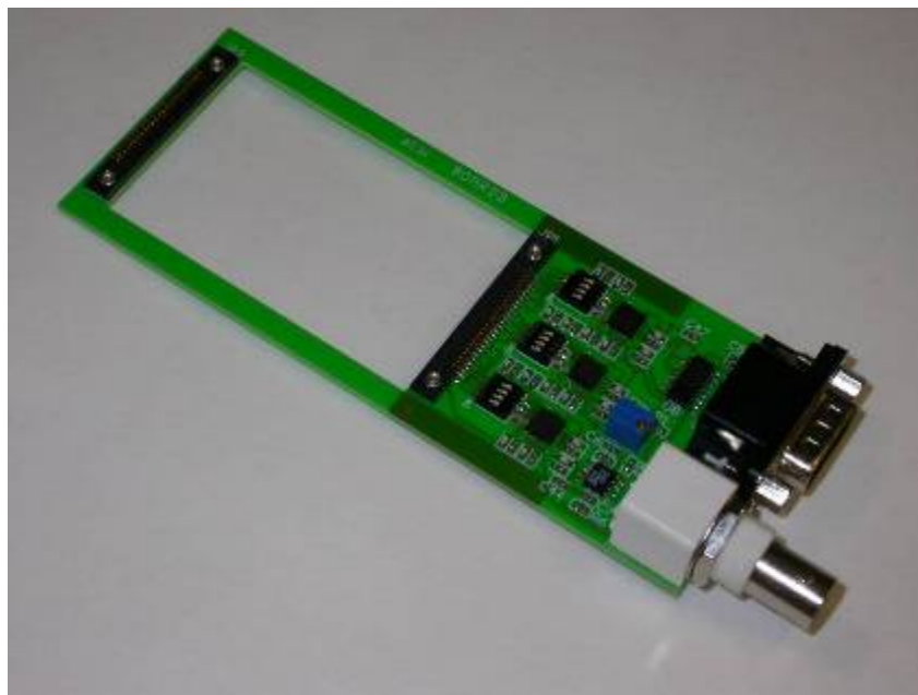
Figure 26: Three silicon chips have been mounted using a SMT technology in a board to be interfaced with microfluidic structure that needs to be inserted in the left aperture.
